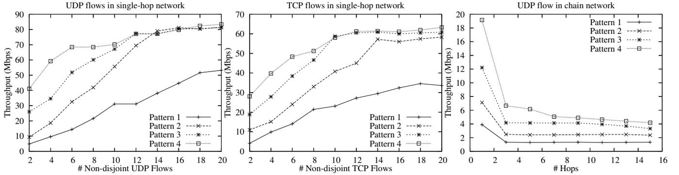
Figure 3: Network throughput achieved by b-SMART in different fragmentation patterns
