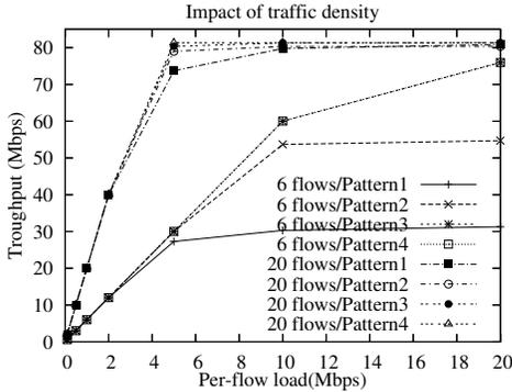
Figure 4: b-SMART adapts to varying traffic patterns to use all the available bandwidth
