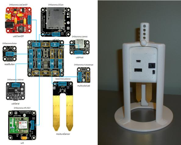
**Figure 1.** .NET Gadgeteer modules (left) and encased prototype (right) for moisture sensor
