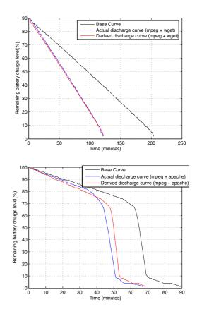
Figure 7. Base curve together with discharge curves (actual and derived) for the new HP laptop (top) and old Dell laptop (bottom)
