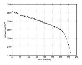
Figure 3. Base curve for an HP iPAQ
