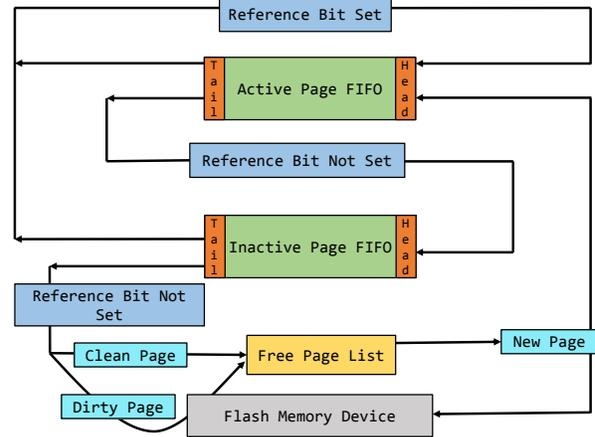
**Figure 3: Chameleon uses two FIFOs to track activity of SVMPs instead of pages**
