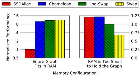
**Figure 8: Searching workload – testing in-memory and out-of-core graph traversal performance of the three systems.**
