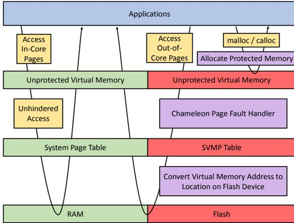
**Figure 4: Overview of how Chameleon services a page fault triggered when application accesses a page on flash. Pages in RAM are freely available.**
