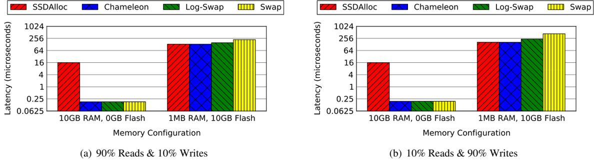
**Figure 5: Microbenchmarks with random reads/writes on 0.5KB objects. Chameleon matches the lowest latency for random accesses under all settings when compared to SSDAlloc and Log-Swap.**
