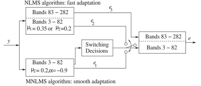
Fig. 1. Proposed dual-structured AEC architecture.
