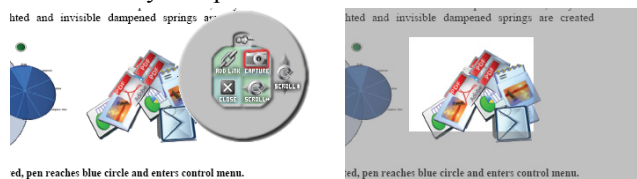
Fig. 11. Using the tracking menu to capture piece of a document. Left: The user taps on the Capture button. Right: A gray mask is applied to the entire screen and the user sweeps out the desired clipping.
