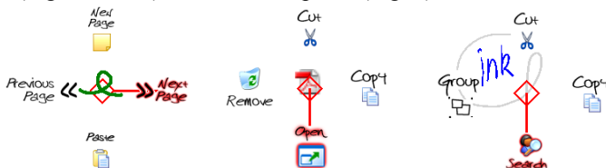
Fig. 6. Left: A pigtail gesture over empty space brings up a menu for the notebook. Center: A stroke starting on an icon opens a marking menu. Right: A pigtail at the end of a lasso activates a context menu.
