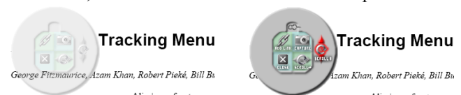
Fig. 10. Tracking menu for document functions. Left: inactive state when pen is not over the menu. Right: active state with pen over the outer ring (“scroll”).
