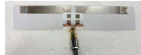
**Figure 4.** This printed antenna was initially resonant at 807 MHz but was adjusted to 920 MHz using a Circuit Eraser to reduce its length. It was then re-tuned to the original resonant frequency with a conductive pen – the manually reworked areas can be seen at each end of the dipole on close inspection.
