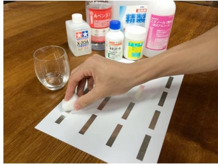
**Figure 2.** We evaluated 4 different materials and 6 different solvents. This is a melamine sponge soaked in alcohol.
