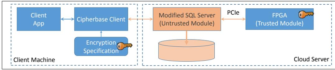
Fig. 3. Cipherbase Architecture
