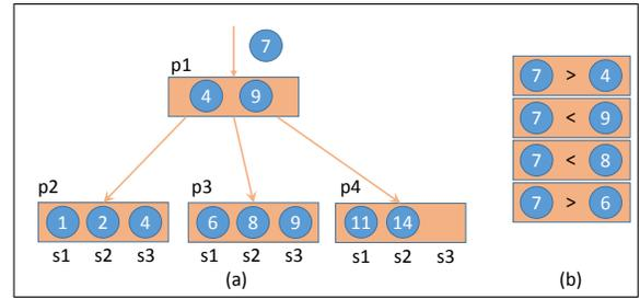
Fig. 5. A single-column range index. Strongly encrypted ciphertext is shown with a blue circle over the plaintext (not visible to the adversary). Page ids ( $p1$ - $p4$ ) and slot ids ( $s1$ - $s3$ ) within pages are also shown. Also shown are comparisons and their plaintext results while inserting (encrypted) key 7. The results of comparisons ensure that key 7 is inserted between keys 6 and 8.
