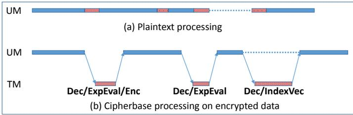
Fig. 8. Transaction processing in Cipherbase involves a large number of fine-grained TM accesses.
