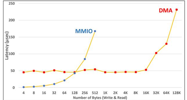
Fig. 7. PCIe Communication. Latency of loopback host/FPGA transfer.
