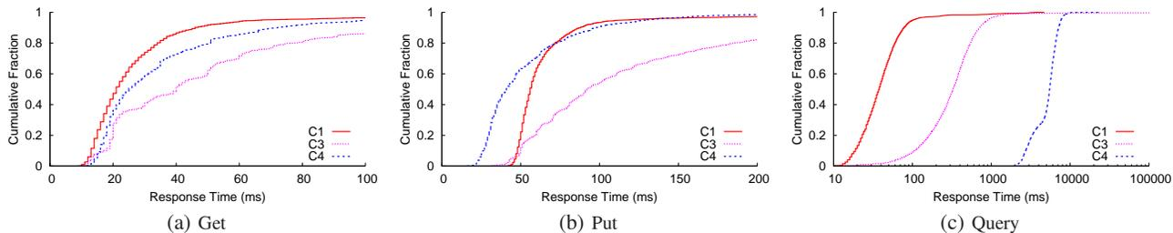
**Figure 4:** The cumulative distribution of the response time when using the large table with 100K entries. Note that for the query operation, the x-axis is in a logarithmic scale, due to the significant performance gaps between different services.
