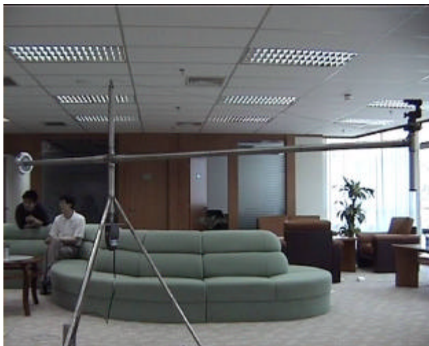
Figure 1: Capturing device of concentric mosaics.
