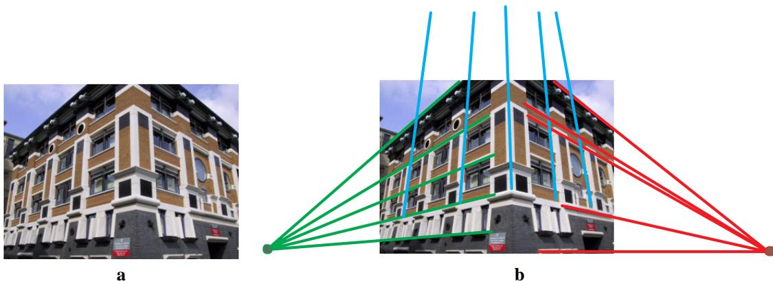
**Figure 1:** In a photograph parallel scene lines are imaged as converging lines. (a) A photograph of a building in Cambridge, UK. (b) Three sets of parallel lines (in green, blue and red) are shown. In the image plane all the lines in each set converge into a single point, namely the vanishing point. The vanishing point associated with the set of lines shown in blue falls well outside the image.
