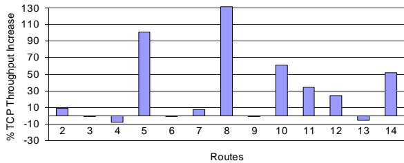
Figure 19: Macrobenchmark: heterogeneous node scenario. TCP throughput gain on paths from node 1 to all other nodes.
