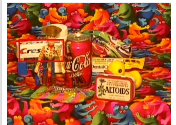
Figure 6: Algorithm finds toothpaste box in spite of partial occlusion and background clutter.
