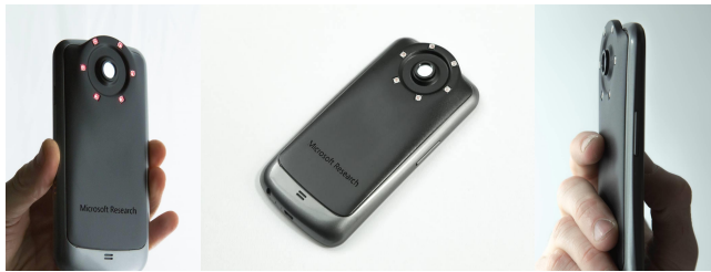
Figure 3: A modified smartphone with additional NIR LED ring, bandpass filter, and custom 3D printed casing.
