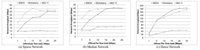
Figure 7. Network throughput vs offered load in ns2 simulation with 54Mbps channel in networks with different density.
