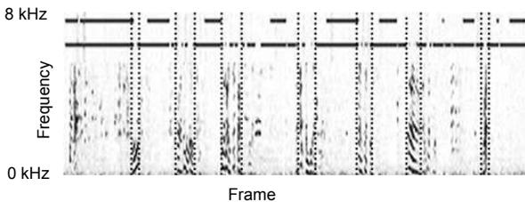
**Fig. 5.** Spectrogram of the AEC+HDRES algorithm output. Segments between dashed lines represent near-end speech. The bars indicate single-talk segments with (upper) and without (lower) double-talk detector enhancements.
