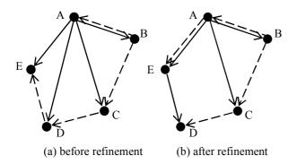
Fig. 2. An example of the multicast tree adjustment in the refinement algorithm
