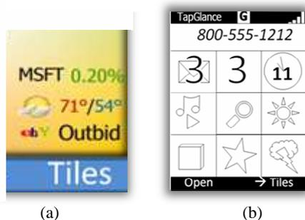
**Figure 4: TapGlance scales to different audiences: (a) full color with text at 320x240 and (b) black and white with icons at 128x96**
