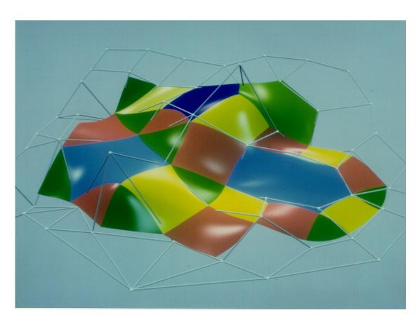
Figure 5.10: A surface with an irregular control net
