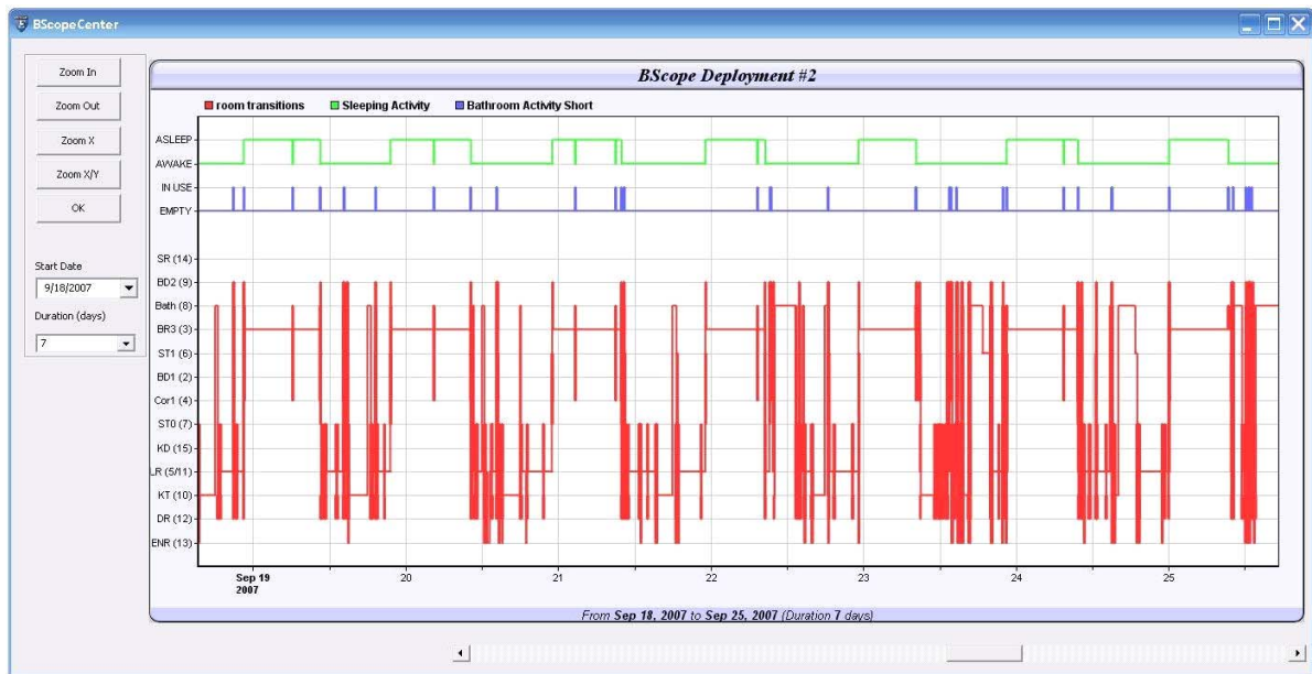
Figure 8: Room transitions and detection of sleeping activity and bathroom usage (using rule based triggers) of the monitored person for a period of one week.
