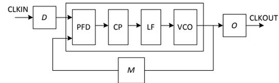
Figure 10. Virtex PLL Structure.
