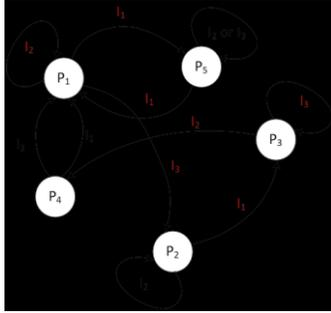
Figure 4. FSM of LTL assertion after state optimization.
