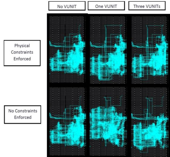
Figure 7. Placement of SIRC with different quantities of assertion cores (VUNIT).
