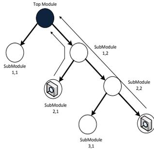
Figure 6. Passing internal signals to top level for probing.
