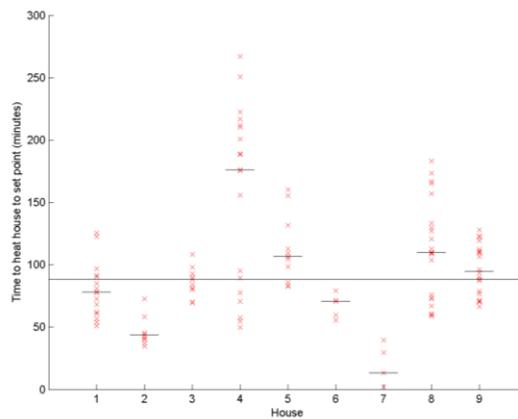
Fig. 5. Heating period durations. Black lines are medians; long black line (overall median) at 88 mins.
