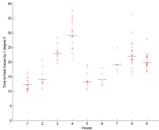
Fig. 4: Heating rates measured in the study for each heating period in each house. Black lines are medians.
