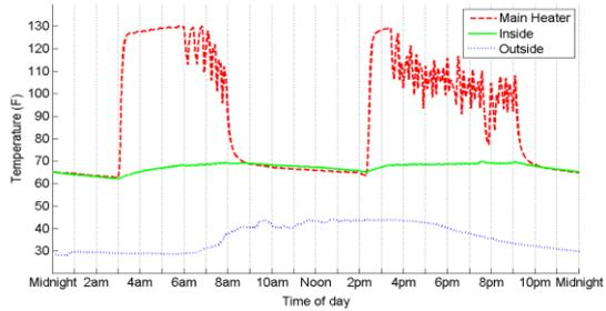
Fig. 3. Temperature record for a single house and day
