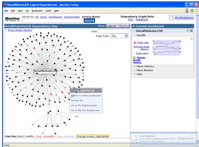
**Figure 1.** Maya in action: the directed graph visualizes the system components, their health (red/black), and the dependencies between them. The square in the top-right corner is a dashboard for one of the components showing the most important metrics, alarms, and other information.
