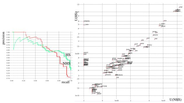
Figure 3: Hierarchial Feature Extraction. Precision-recall performance (left) and term U-values (right) for the hierarchical (HS) and non-hierarchical (NHS) models (see text for details).
