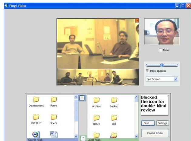
**Figure 2.** The view from the remote person; the upper-center portion is a live view from the meeting room: the person who is talking is shown at the top with high resolution, and the whole meeting room is shown at the bottom with low resolution. The upper-right portion shows the video of the local person him/herself. The bottom portion shows the UI for file sharing and transfer.
