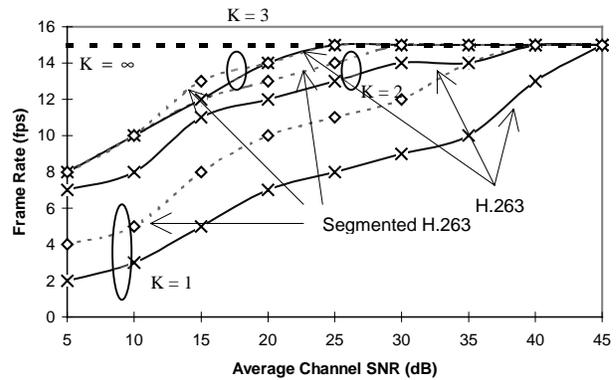
Figure 7: Comparison of temporal resolution with changing error characteristics
