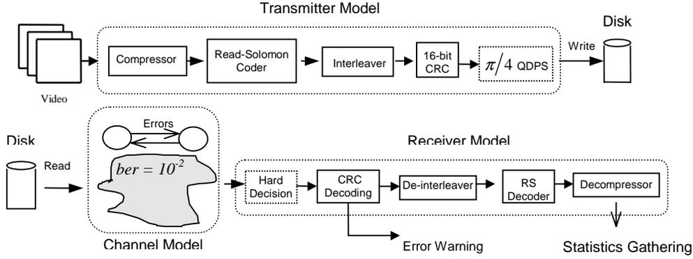
Figure 1: Simulation architecture for studying the performance of video over radio channels
