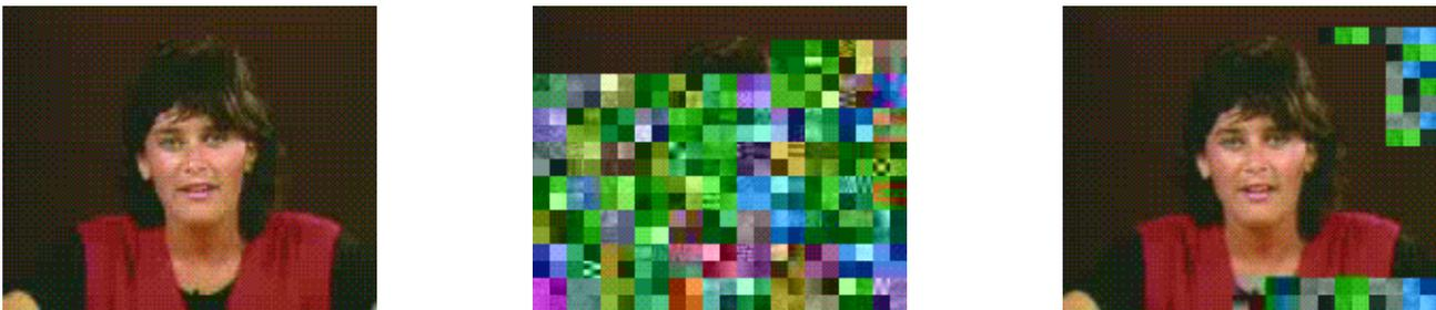
Figure 5: Example of error propagation containment with region segmentation
