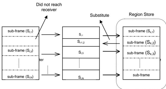
Figure 3: Reconstruction of a video frame
