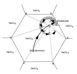
Fig. 2. Geometry for calculating cell-crossing probability
