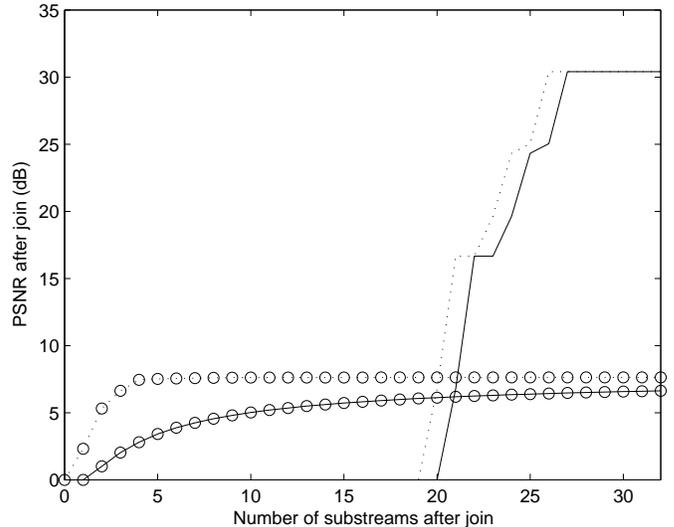
Fig. 2. Join Experiment for RLM vs. MDC: no collateral damage in MDC
