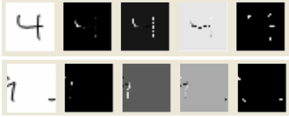
Figure 5. The left most images in each row are the candidate and context images rendered at 29x29 pixels. The remainder of each row shows various feature images computed from these principle images. From left to right: stroke curvature, stroke normal X, stroke normal Y, and endpoints.
