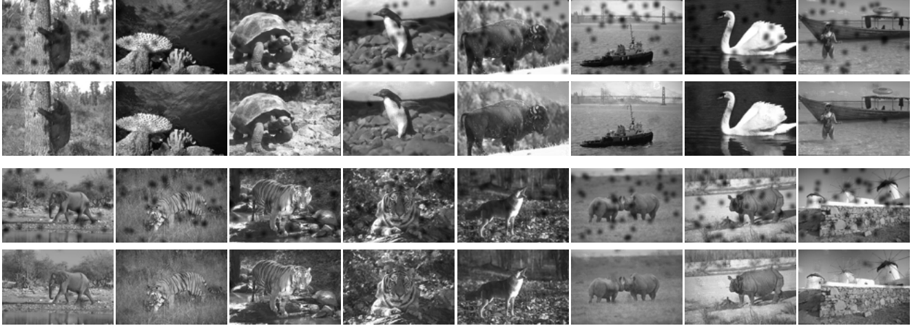
Figure 5. Additional representative test set results for image denoising with structured noise. First and third row: input images with simulated dust on the camera lens. Second and last row: RTF denoising results with a 3x3 model and decision trees of depth ten (PSNR 27.85).
