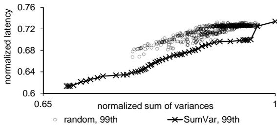
**Figure 9:** This plot shows the results of a random search in the reissue budget space (circles) and using SumVar on the same workflow (line with crosses). It illustrates that as sum of variances (x-axis, normalized) decreases, so does the 99<sup>th</sup> percentile of latency (y-axis, normalized).
