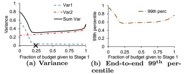
Figure 2: Impact of splitting the budget between two stages in a serial workflow on the variance of individual stages (Var1 and Var2), and the variance (Sum Var) and 99<sup>th</sup> percentile of the end-to-end latency (metrics are normalized)
