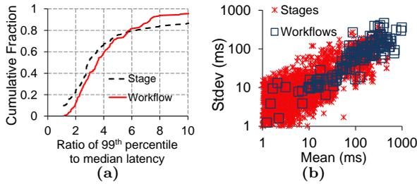
Figure 4: Estimating the variability in latency: (a) CDF of 99<sup>th</sup> percentile to median latency and (b) mean vs. standard deviation of latency, for stages and workflows.
