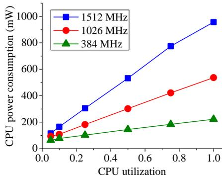
**Figure 2: Power consumption of a single Nexus 4 CPU core at different CPU utilizations.**
