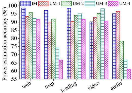
Figure 9: Single-core model accuracy with real apps.
