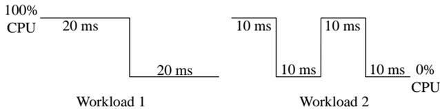
**Figure 1: Two periodic workloads with the same CPU utilization (50%) but different CPU usage patterns.**
