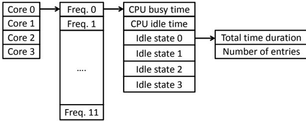
**Figure 6: Data structure used in the data collector.**
