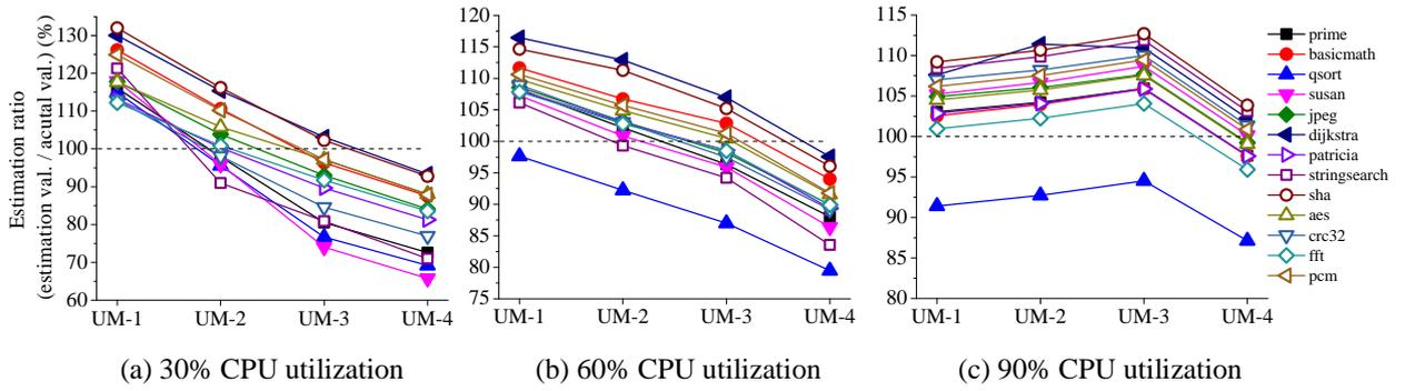
Figure 8: Estimation ratios of the four utilization based models (single-core).
