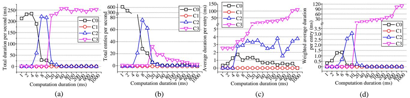
**Figure 4: Single-core power model development.** Figures (a)-(d) show  $T_{C_i}$ ,  $E_{C_i}$ ,  $ED_{C_i}$ , and  $WED_{C_i}$  for the four CPU idle states  $C_0 - C_3$ , respectively (with CPU frequency  $f = 1,512$  MHz, utilization  $U = 75\%$ ).
