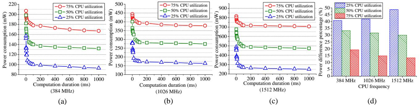
**Figure 3: Workloads running in multicore CPU with the same CPU utilization and frequency consume notably different amounts of CPU power.**
