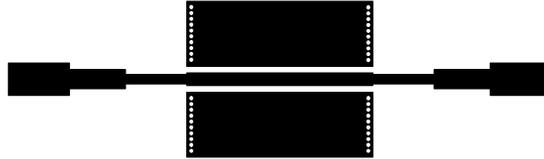
Fig. 4: A top view of the test circuit layout which includes the CPW and microstrip TL. This circuit has a 360 degree phase shift at  $d=0$  mm. The bottom layer of the CPW section does not have a ground plane and *via* is used for connecting the ground.
