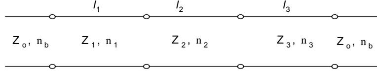
The non-enhanced section is given by  $Z_0$  and  $n_b$ . The center sections will be enhanced, and they are given by  $(Z_1, n_1)$ ,  $(Z_2, n_2)$  and  $(Z_3, n_3)$  where  $Z$  and  $n$  are characteristic impedance and the index of refraction of each section. We want to create impedance matching for all states. This can be done by satisfying the following conditions:
