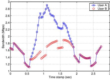
**Figure 10:** The network throughput of interactive delivery. Red curve is the network throughput of a single view stream, and the blue curve is that of a clip containing a frozen moment effect.
