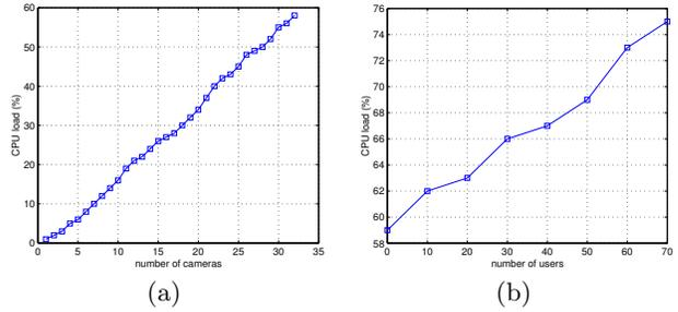
**Figure 11:** (a) Computational cost vs. number of cameras. (b) Computational cost vs. number of users.
