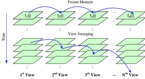
**Figure 2: Examples of visual effects provided by multi-view video** ( $f_n(i)$  denotes the  $i^{th}$  frame of the  $n^{th}$  view).
