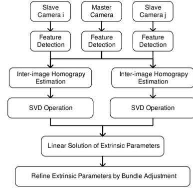
**Figure 3: The pattern free calibration.**
