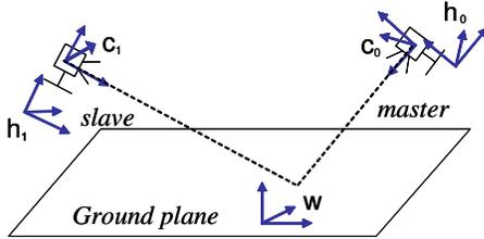
**Figure 4: Master-Slave Tracking.**  $w$  is the world coordinate system,  $h_0$  and  $h_1$  are the hand coordinate systems, and  $C_0$  and  $C_1$  are the camera coordinate systems.
