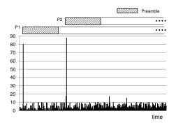
Figure 11: Detection of a preamble. The cross-correlation result of two measured overlapped frames transmitted at 1MBs with a  $20\mu s$  sample template of preamble.
