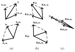
Figure 7: Illustration of interference nullifying.
