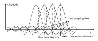
Figure 2: Symbol timing offset and inter-symbol interference.
