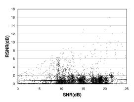
Figure 14: Performance of interference nullifying. The solid line plots the linear regression of the data.
