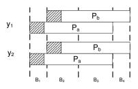
Figure 10: The tracking mode of chain-decoding. A long frame is divided into blocks. Chain-decoding decodes each block sequentially. The decoded symbols are then used for updating the symbol timing and frequency offset.
