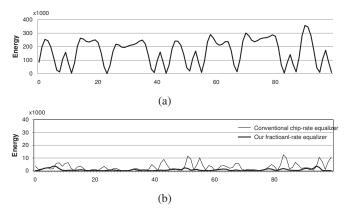
Figure 9: Equalization for interference nullifying in multi-path fading channel. IN is performed on a single frame transmitted to two receiving antennas. (a) Original interference signal. (b) The nullifying results with the conventional equalizer and our extended equalizer design.
