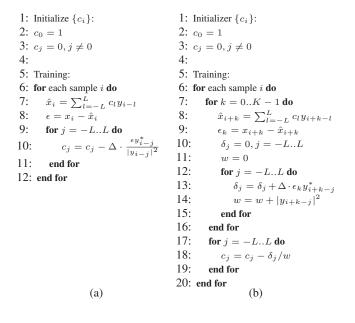
Figure 8: Pseudo-code for equalizer training algorithms. The same algorithm also applies to channel estimation with the exchange of input and output.
