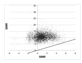
Figure 16: Performance of interference cancelation. The x-axis shows SINR of the first frame before IC; the y-axis shows SINR after IC. The solid line shows the "y=x" line.
