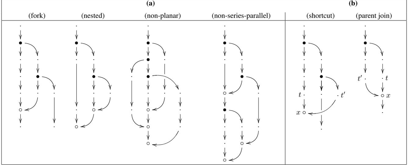
**Figure 1.** (a) Four examples of revision diagrams. (b) Two diagrams that are not revision diagrams since they violate the join property at the creation of the join node  $x$ . In the rightmost diagram,  $F(t')$  is undefined on the main revision and therefore  $F(t') \rightarrow^* t$  does not hold.
