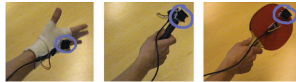
Figure 2. IMU placement in each of the Prop Fidelity conditions: on the back of the palm for the hand, and on the tip of the prop for both the stick and the paddle.
