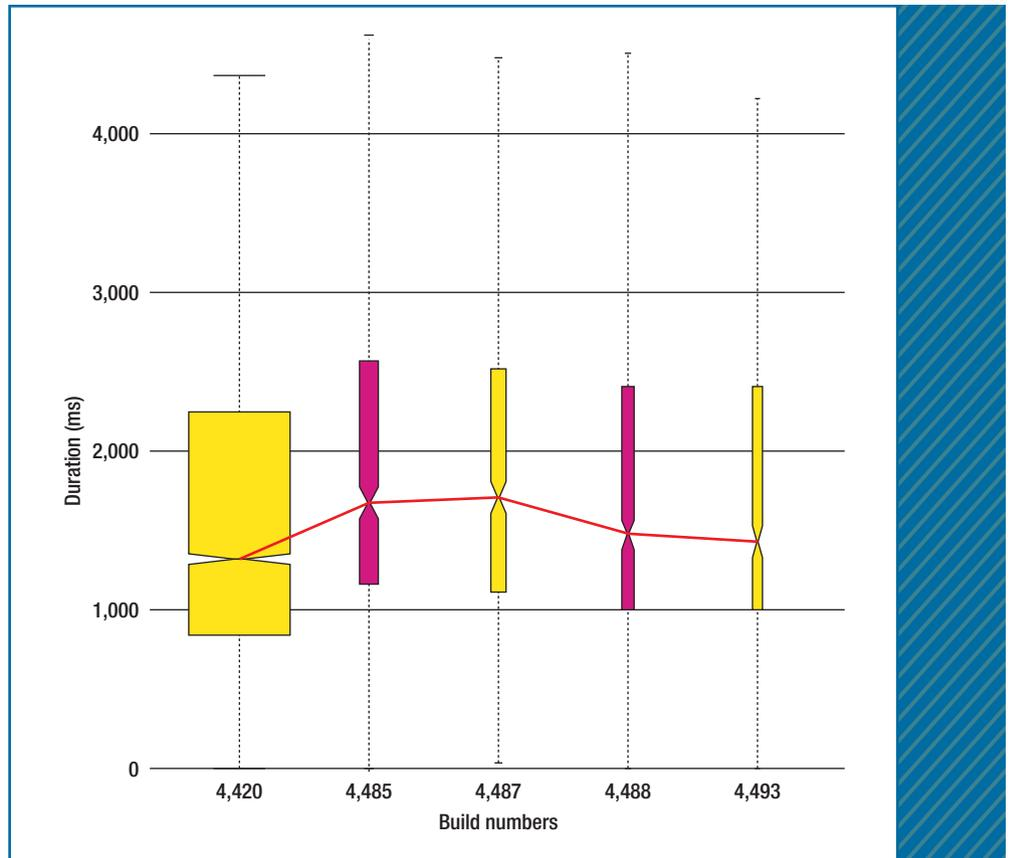
**FIGURE 4.** A build-over-build analysis. Red indicates a statistically significant difference from the previous build. Width indicates the number of users who used this scenario for this build. Height shows the interquartile range.
