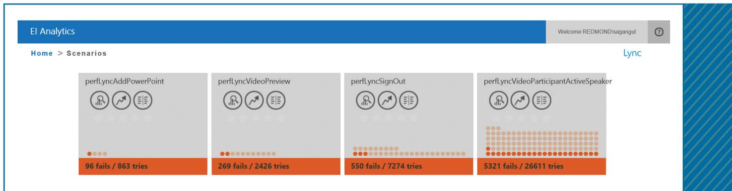
**FIGURE 1.** A sample of high-level view results for four scenarios in Lync. In each cell, the color reflects the overall prognosis (gray is untested; red and green show performance levels). The fails summary provides the number of attempts that didn't succeed; the other buttons lead to various visualizations and detailed reports on the scenario.
