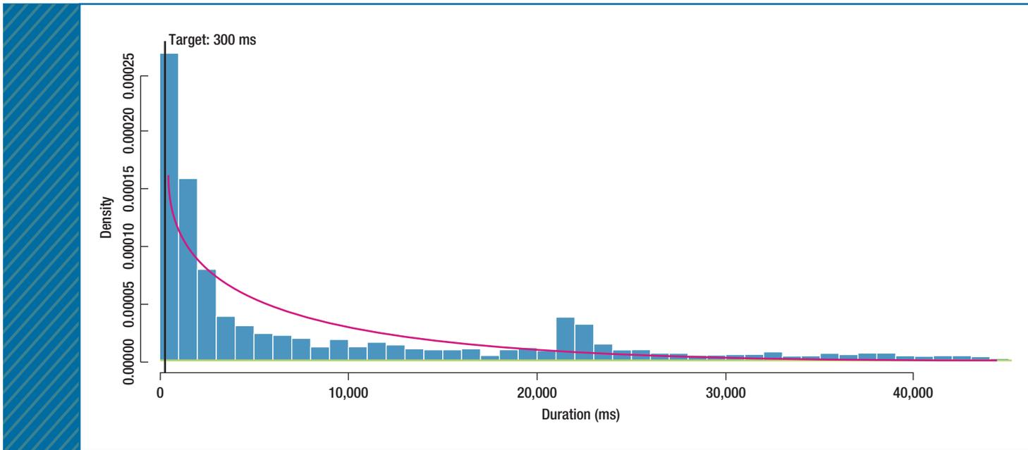
**FIGURE 6.** A histogram of durations for a scenario for a given build. Note the peak around 21,000 milliseconds, which alerted testers to an IPv6 timeout defect that didn't manifest in standard testing.
