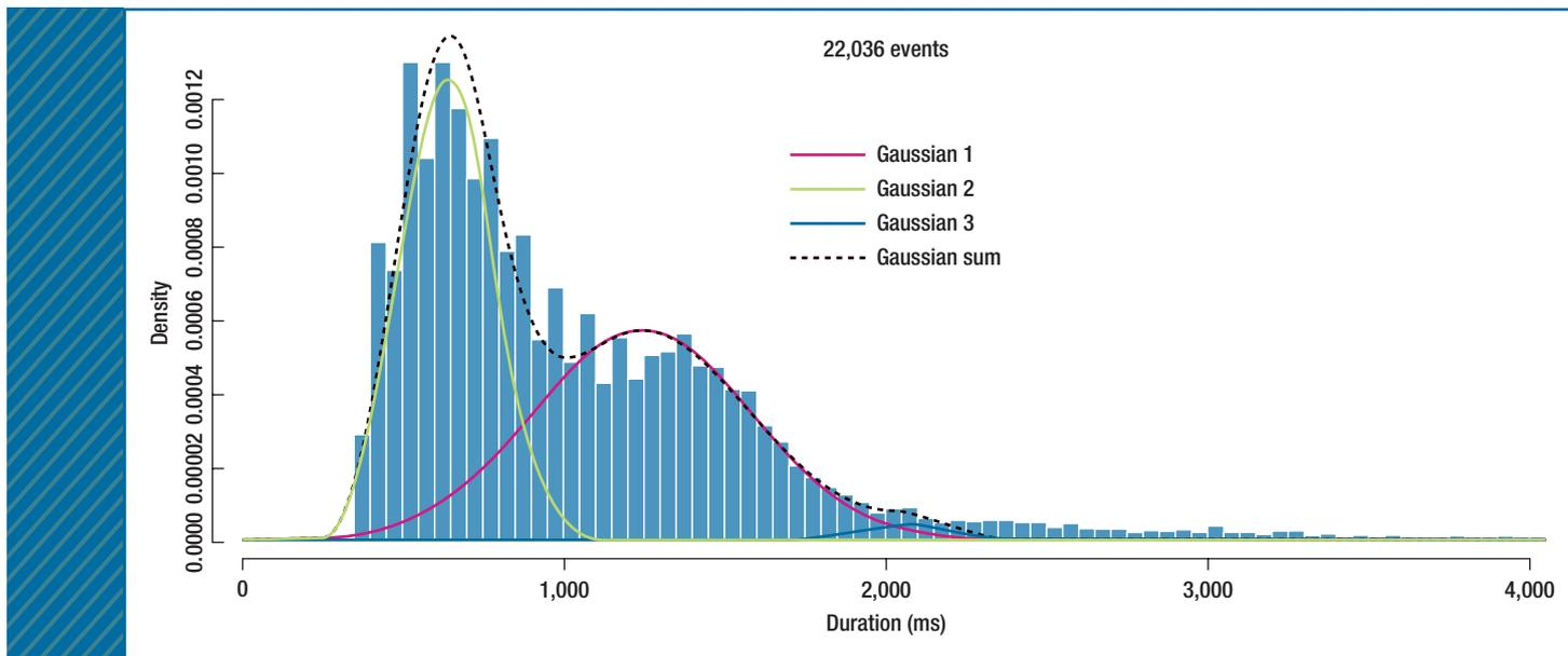
**FIGURE 2.** A histogram of the durations for a single scenario for a given build. The durations are fit to the sum of Gaussians, which each represent a different user experience.
