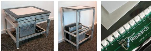
**Figure 4:** (i) Table in its collapsed state, (ii) ready for use, and (iii) close up of edge lit IR LED illumination, acrylic sheet, latex sheet and drafting film.
