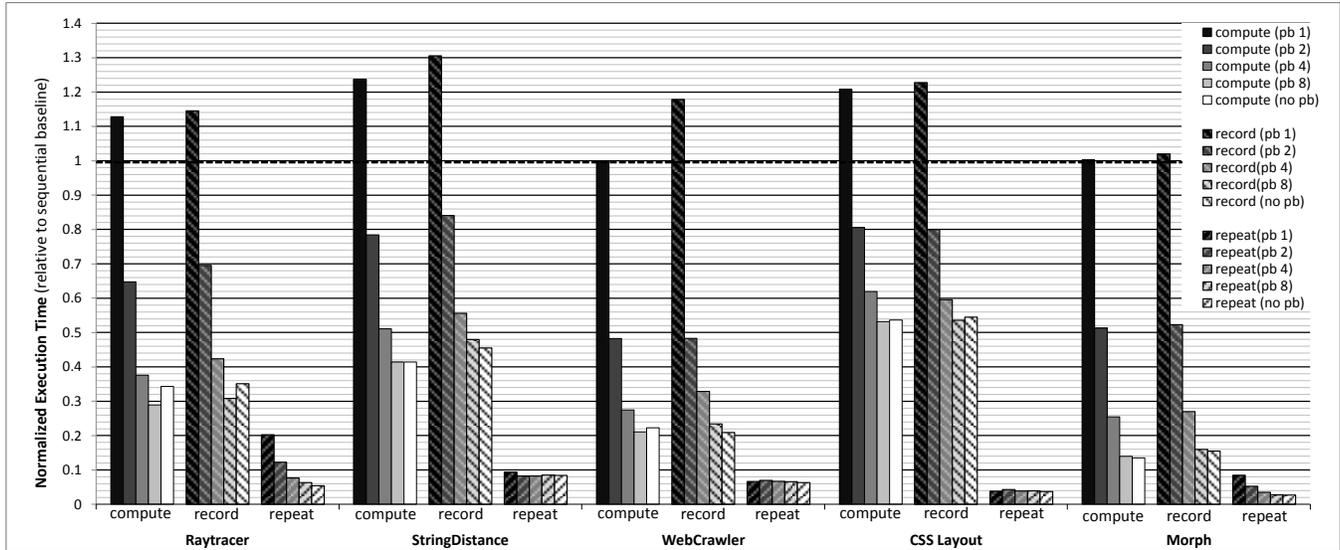
**Figure 12.** Graphical representation of normalized execution times for compute, record and repeat, relative to the sequential baseline. Lower is better. We show execution times for various parallelism bounds (for example, pb=4 instructs the revision scheduler to schedule at most 4 revisions in parallel).
