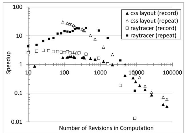
**Figure 14.** Effect of the granularity on speedups. The horizontal axis shows (on a logarithmic scale) the number of revisions in the computation (which increases exponentially when we decrease granularity). The vertical axis shows the speedup (or slowdown, if less than 1) relative to the baseline, also on a logarithmic scale.
