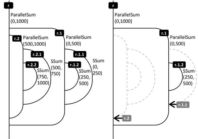
**Figure 3.** Revision diagrams illustrating the initial computation recorded by `record` (left) and the repeated computation performed by `repeat`. On repeat, the runtime avoids reexecuting some of the revisions, and simply replays their effects on join.
