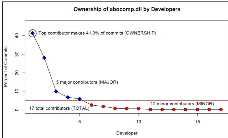
Fig. 1: Graph of the proportion of commits to `abocomp.dll` by developers during the Vista development cycle, showing the four measures of ownership used in this paper.
