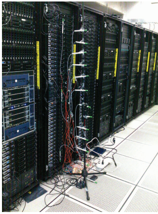
Figure 2: A picture of the air flow sensors setup. We positioned 12 air flow sensors directly above the floor vent at a vertical interval of 5.25", or every 3U.
