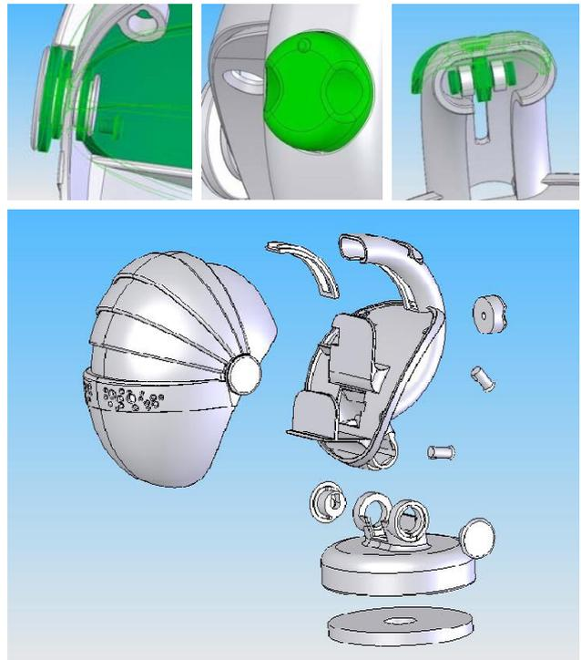
Fig. 11. The 3D modelled additional features and an exploded view of all the separate components.
