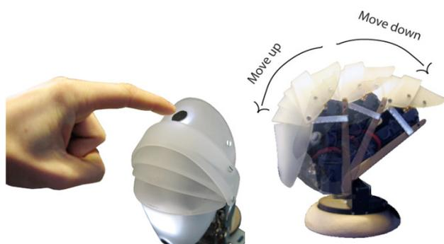
Fig. 6. Interactive buttons; tap makes object move up or down.
