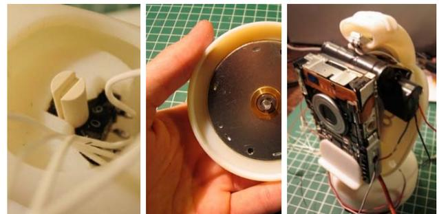
Fig. 12. The integration of the electronics in the printed parts.
