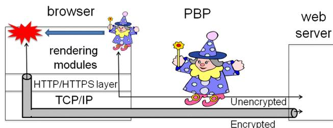
Figure 1. PBP attacks the encrypted data after they are decrypted above the HTTPS layer
