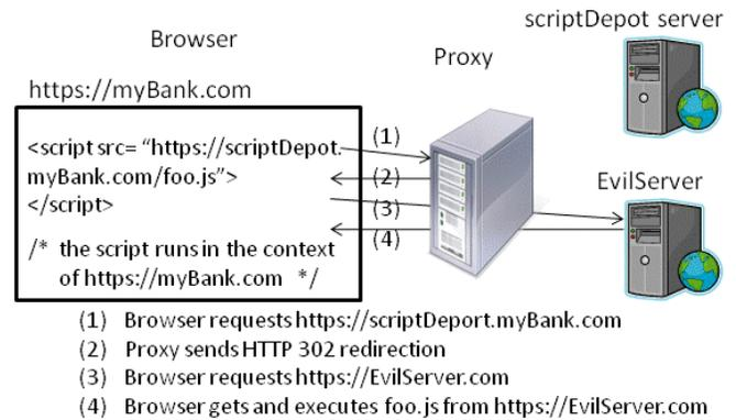
Figure 3. The attack using 3xx redirection message
