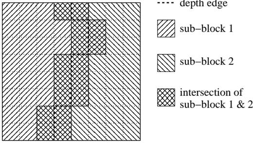
Fig. 3. Example of overlapping motion compensation.
