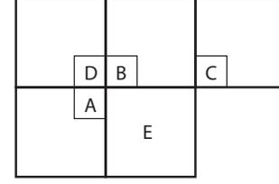
Fig. 4. Motion vector prediction for E is the median value of A, B and C or D depending on position.
