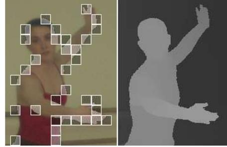
**Fig. 2.** Example of  $z$ -mode MBs for Ballet sequence in high-bitrate: segmentation of texture MBs around boundary of dancer into sub-blocks (left) using corresponding depth data (right).
