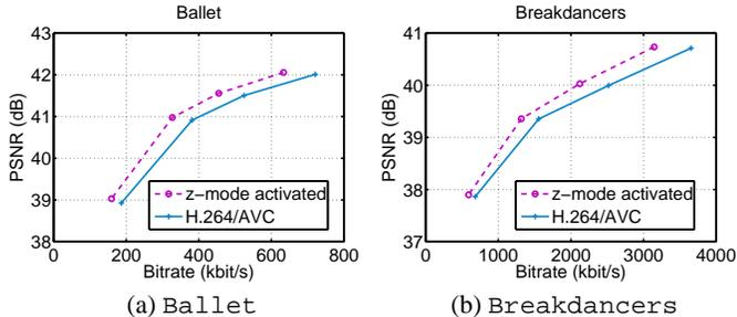
Fig. 5. Objective PSNR results of texture coding.
