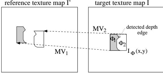
**Fig. 1.** Motion compensation of sub-blocks in texture map divided using detected edge in depth map.
