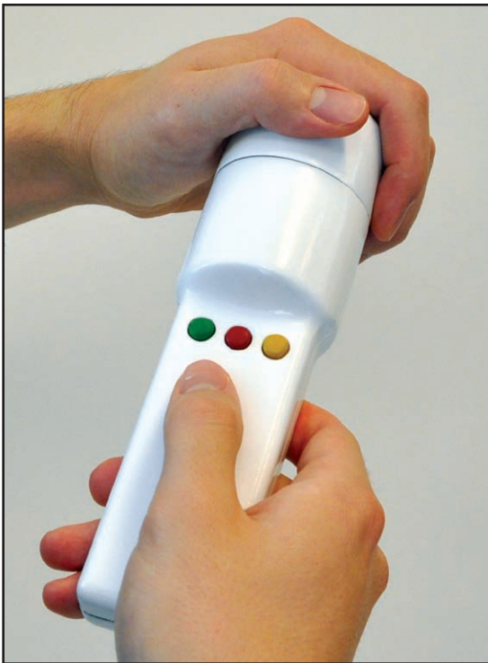
Figure 3. The Peppermill is a general-purpose wireless input device that derives both power and control information from manual rotary input.
