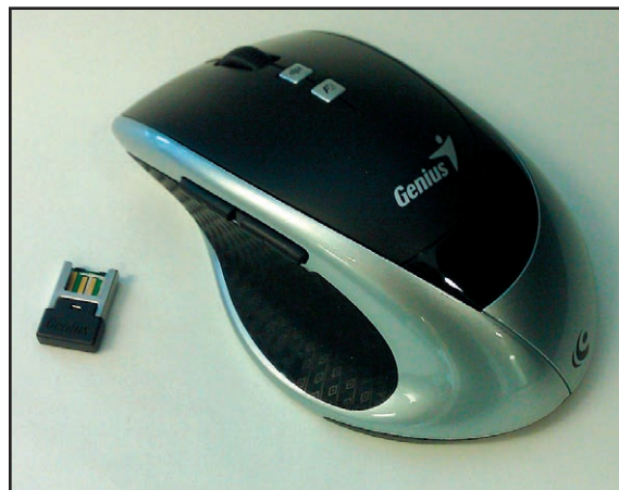
Figure 1. The Genius DX-ECO wireless mouse uses a supercapacitor instead of batteries, enabling ultrafast recharging.
