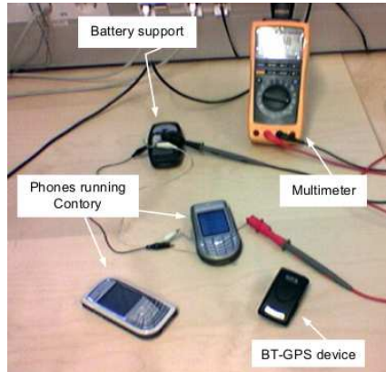
Fig. 3. Power measurements testbed setup
