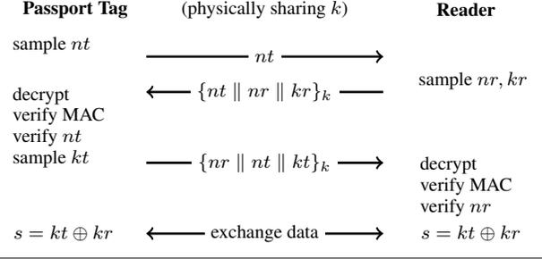
**Figure 1.** Basic Access Control protocol for passports
