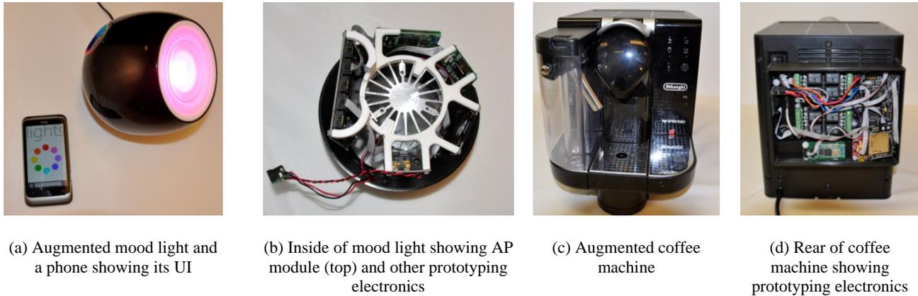
**Figure 1. Prototype appliances supporting phone web UIs (SAWUIs). Much of the extra electronics could be eliminated in production devices. SAWUIs employ HTML, CSS & JavaScript served by a webserver and WiFi access point in the appliance.**
