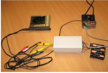
Figure 3: SenseCam with video logging hardware
