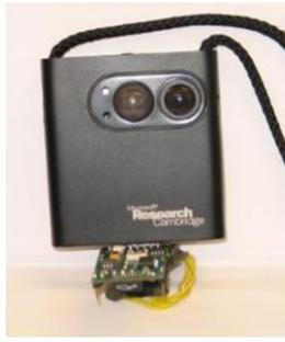
(a) SenseCam with added compass sensor
